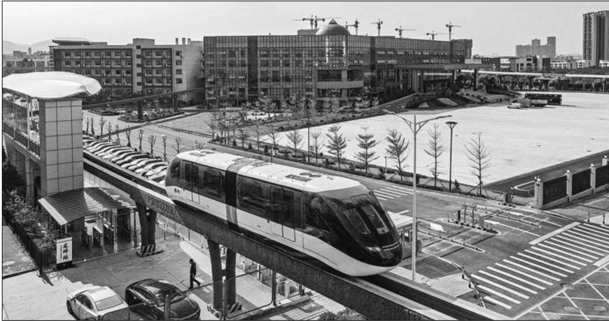
An electric train runs on BYD's Cloud Rail, a straddle-type monorail, at the company's headquarters in Shenzhen, Guangdong province, in February. ZHU HONGBO / FOR CHINA DAILY
