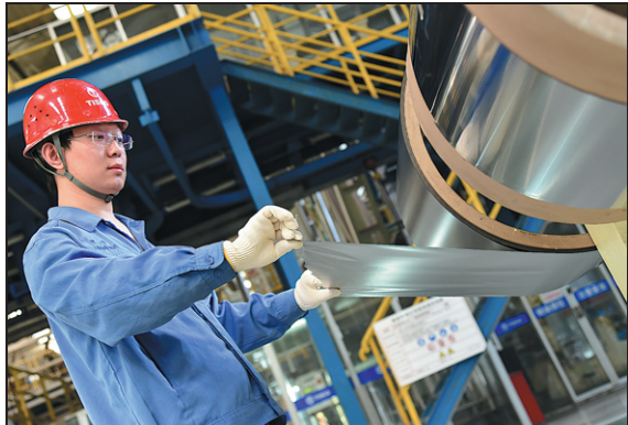
With a thickness of 0.02 millimeters, the stainless steel foil produced by Taiyuan Iron and Steel is considered a high-end product in the industry. WANG XUHONG / FOR CHINA DAILY
