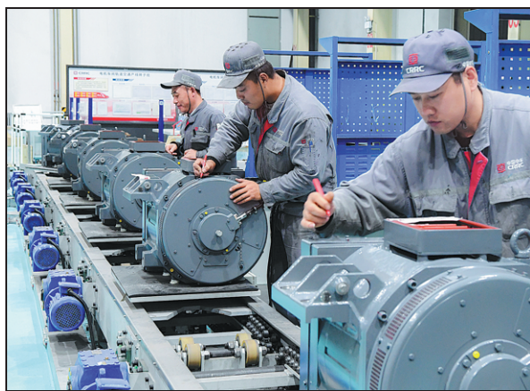
Staff members of CRRC Yongji Electric Motors assemble the permanent magnet traction motors to be used in the new-generation bullet train which has a top speed of 400 kilometers per hour. DAI CHENKAI / FOR CHINA DAILY
