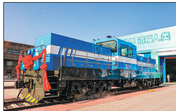
China's first independently developed hydrogen fuel-cell hybrid locomotive rolls off the production line at CRRC Datong. WANG PEI / FOR CHINA DAILY
