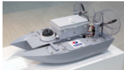
A (boat type) robot for examination of concealed culvert leakage, theft of concealed pipes, concealed culvert blockage and other situations
