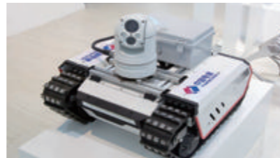
A (tracked) robot for video detection of illegal discharge in urban culverts in the absence of water or with a small amount of water
